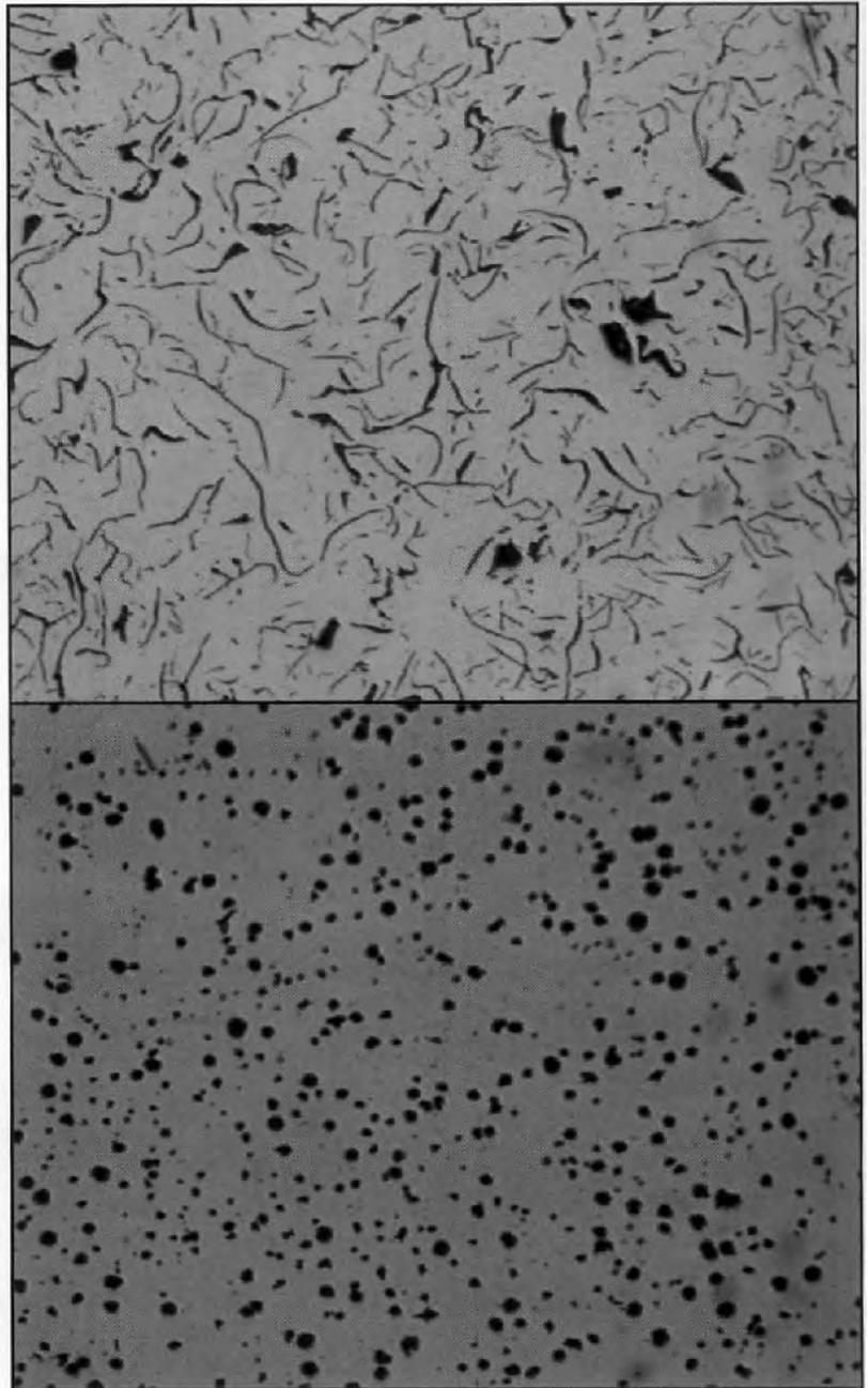
Fig. 1 - Flake (top) versus nodules (bottom) graphite cross sections.
