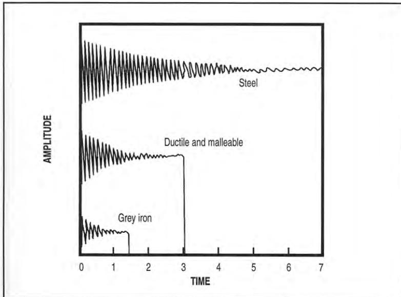
Fig. 2 - Relative damping behaviors of steel, ductile & malleable irons and gray iron.
